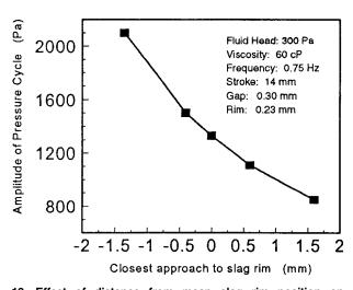
13 Effect of distance from mean slag rim position on slag pressure: slag consumption was reduced to zero as the rim entered the gap (closest approach to slag rim <0)
