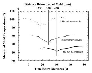
7 Thermocouple measurements showing effect of a transverse depression on temperature drops at successive distances down the mould
