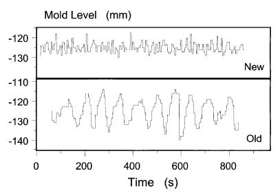
16 Comparison of mould level fluctuations obtained with the old and new control systems for strands C and A respectively
