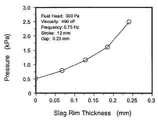
14 Effect of slag rim thickness on magnitude of pressure oscillation
