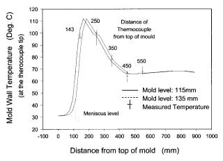
9 Predicted mould temperature profiles for a 20 mm change in mould level
