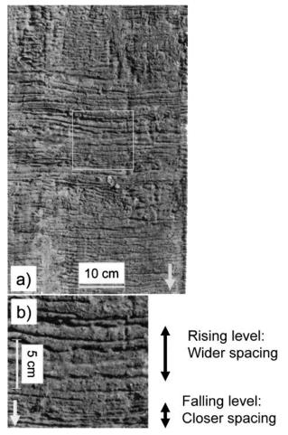
1 a variation in oscillation mark profile and pitch caused by gradual meniscus level variations and b close-up: arrow indicates casting direction
