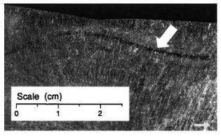
Sub-surface structure beneath a bloom depression: note the faint dark bands that indicate shell thinning as a result of the local reduction in cooling rate caused by the depression
