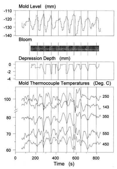
8 Photo of a bloom showing defects highlighted by chalked circles (centre) matched with the corresponding mould level history (top) and the thermocouple temperature profiles (bottom): the latter data has been shifted in time, according to casting speed and distance from the top of the mould, to the same reference point; the measured surface profile is also given (centre)
